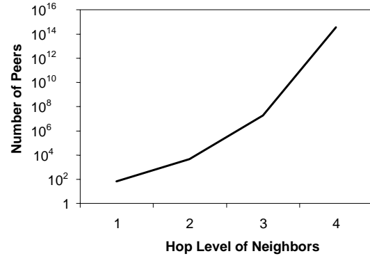
Figure 3. The graph above was plotted using a log Y-axis. It shows how the number of peers that can be reached increases with greater depth. The experiment involved a 10,000 node P2P network. (See Appendix for technique used to form P2P networks)
